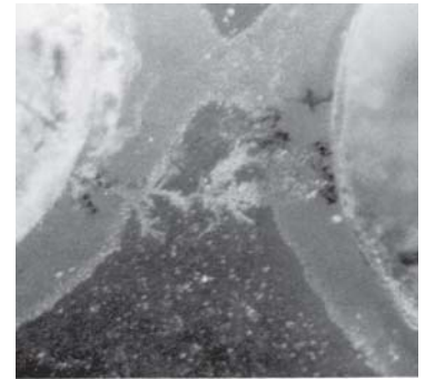
FIGURE 8. Shown - Dendrite corrosion caused by excessive use of a circuit cooler.
