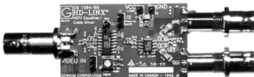
Fig. 34 Photograph of GS1504/GS1508 Evaluation Board
