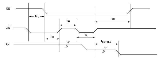
FIGURE 2. SERIAL INTERFACE TIMING DIAGRAM, DECREMENT
