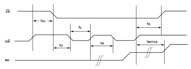
FIGURE 1. SERIAL INTERFACE TIMING DIAGRAM, INCREMENT
