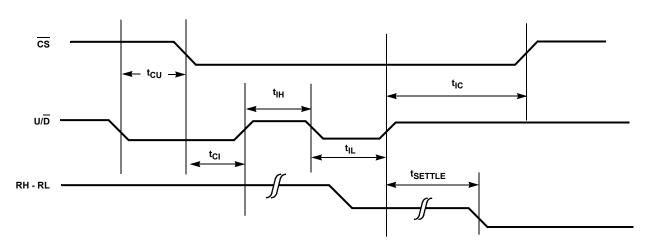
FIGURE 2. SERIAL INTERFACE TIMING DIAGRAM, DECREMENT
