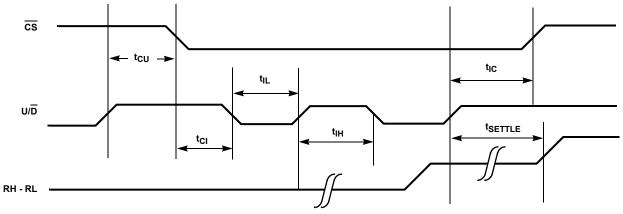
FIGURE 1. SERIAL INTERFACE TIMING DIAGRAM, INCREMENT
