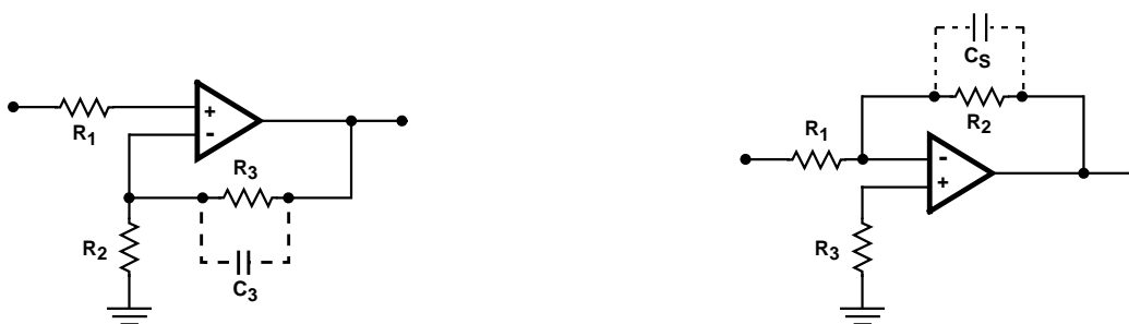
FIGURE 3. SUGGESTED OFFSET VOLTAGE ADJUSTMENT
