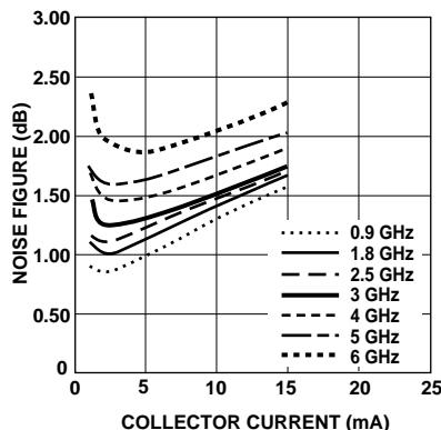
Figure 4. Noise Figure vs. Collector Current and Frequency at 2 V.
