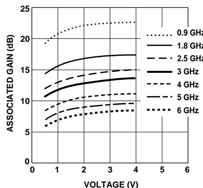
Figure 5. Associated Gain vs. Voltage (V<sub>CE</sub>) at 5 mA.
