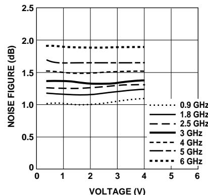
Figure 6. Noise Figure vs. Voltage (V<sub>CE</sub>) at 5 mA.
