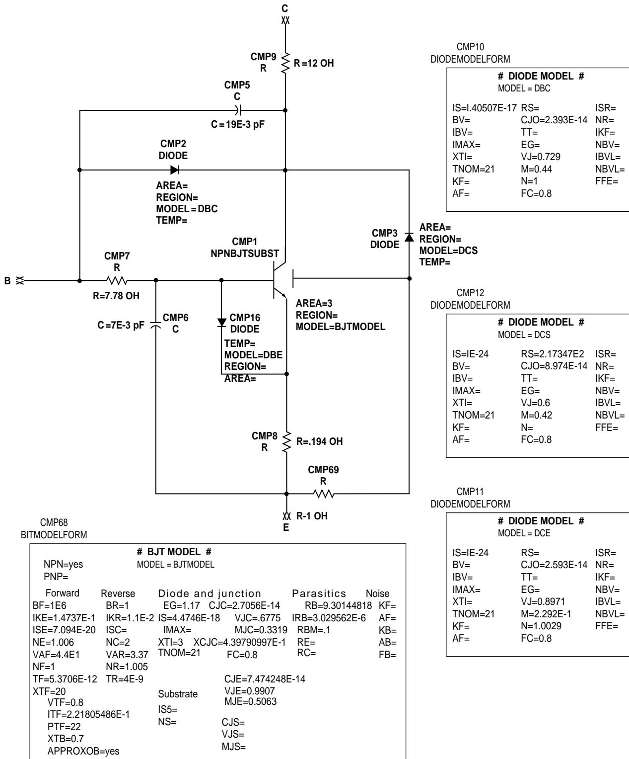
This model can be used as a design tool. It has been tested on MDS for various specifications. However, for more precise and accurate design, please refer to the measured data in this data sheet.
