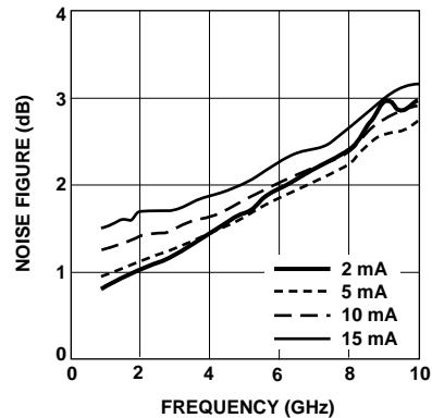
Figure 2. Noise Figure vs. Frequency and Collector Current at 2 V.
