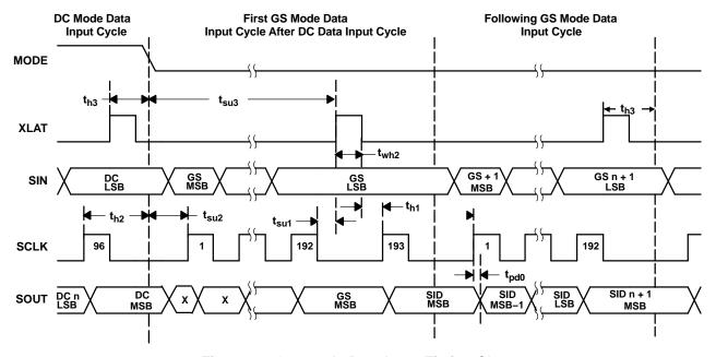
Figure 10. Grayscale Data Input Timing Chart
