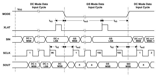
Figure 6. Serial Data Input Timing Chart
