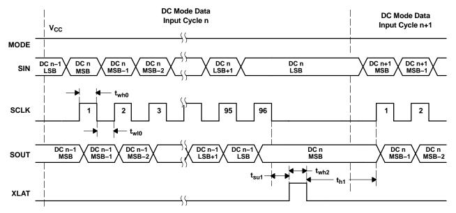
Figure 8. Dot Correction Data Input Timing Chart
