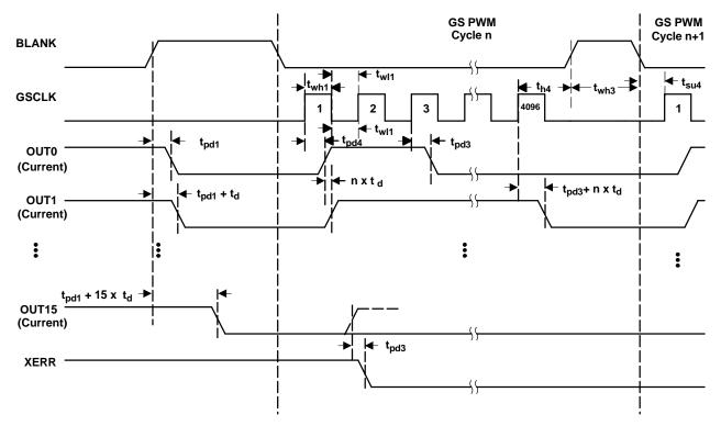
Figure 12. Grayscale PWM Cycle Timing Chart
