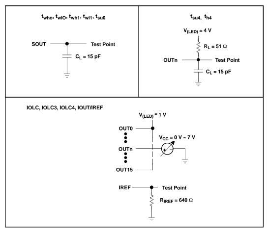
**Figure 2. Parameter Measurement Circuits**
