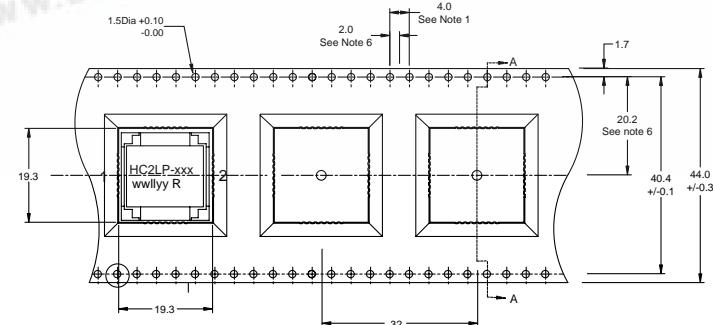
Parts packaged on 13" Diameter reel, 130 parts per reel.
