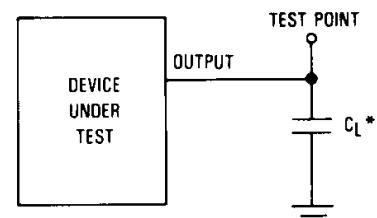
\* includes all probe and jig capacitance.
