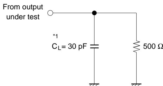
Note: 1.  $C_L$  includes probe and jig capacitance.
