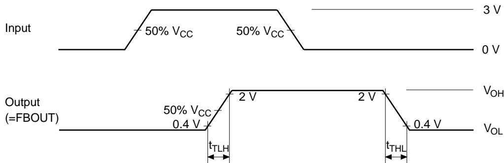
Notes: 1. All input pulses are supplied by generators having the following characteristics:  $PRR \leq 100 \text{ MHz}$ ,  $Z_O = 50 \Omega$ ,  $t_r = 1.2 \text{ ns}$ ,  $t_f = 1.2 \text{ ns}$ .
