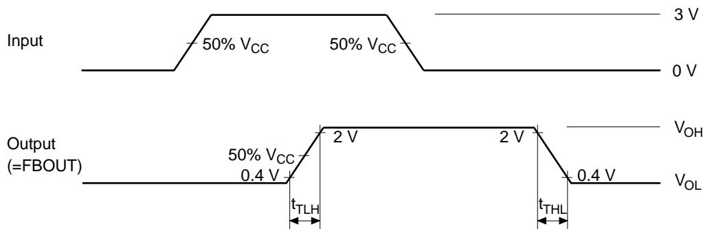
Notes: 1. All input pulses are supplied by generators having the following characteristics: PRR  $\leq 100$  MHz,  $Z_0 = 50 \Omega$ ,  $t_r = 1.2 \text{ ns}$ ,  $t_f = 1.2 \text{ ns}$ .
