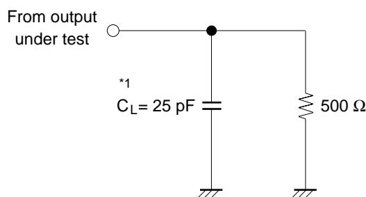
Note: 1.  $C_L$  includes probe and jig capacitance.
