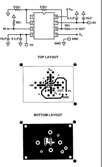
FIGURE 1. EVALUATION BOARD SCHEMATIC AND LAYOUT
