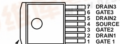
HIP0061AS2 (SIP - GULLWING) TOP VIEW
