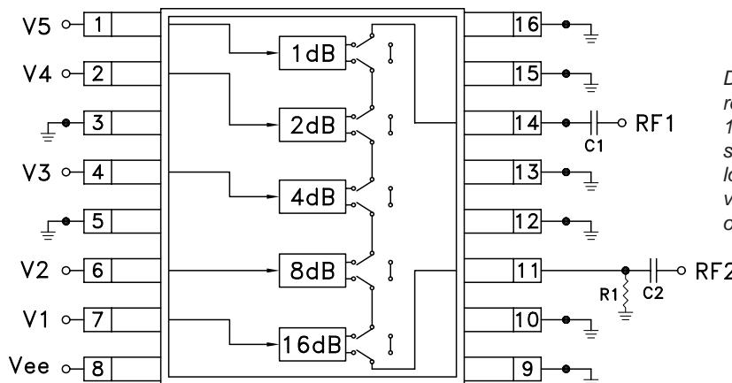
DC Blocking Capacitors C1 & C2 are required on RF1 & RF2. Choose C1 = C2 = 100 pF ~ 0.1 uF to allow lowest customer specific frequency to pass with minimal loss. R1= 5K Ohm is required to supply voltage to the circuit through either Pin 11 or Pin 14.
