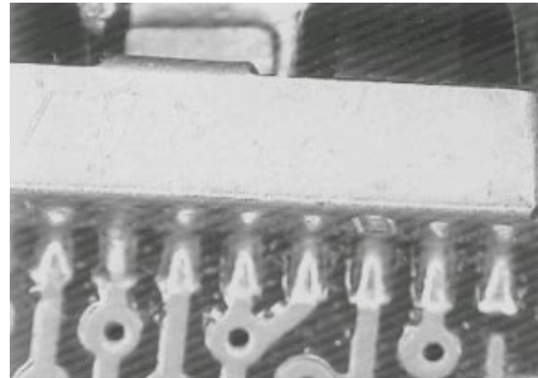
Photo 4.0. Unit self-aligns after reflow.
