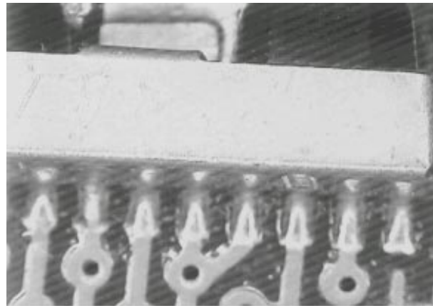
Photo 4.0. Unit self-aligns after reflow.
