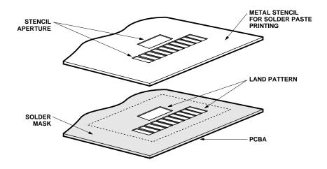
Figure 1. Stencil and PCBA.
