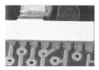
Picture 3. Unit is rotated before reflow.
