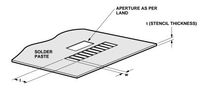
Figure 4. Solder paste stencil aperture.
