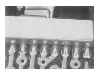
Picture 4. Unit self-aligns after reflow.
