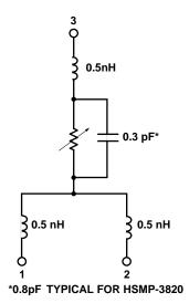
Figure 30. Equivalent Circuit.
