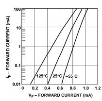
Figure 17. Forward Current vs. Forward Voltage. HSMP-3880 Series.
