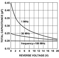
Figure 1. RF Capacitance vs. Reverse Bias, HSMP-3810 Series.
