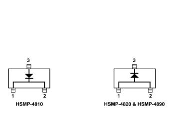
Figure 29. Internal Connections.
