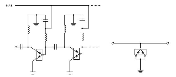
Figure 27. High Isolation SPST Switch (Repeat Cells as Required).
