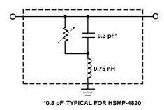
Figure 36. Equivalent Circuit.
