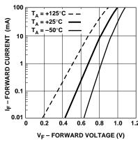
Figure 20. Forward Current vs. Forward Voltage for HSMP-3860.
