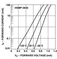
Figure 16. Forward Current vs. Forward Voltage. HSMP-3830 Series.
