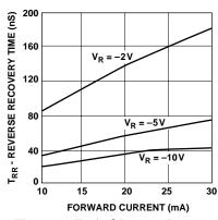
Figure 12. Typical Reverse Recovery Time vs. Reverse Voltage. HSMP-3890 Series.
