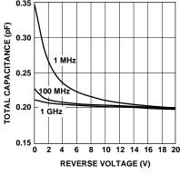
Figure 2. RF Capacitance vs. Reverse Bias, HSMP-3830 Series.
