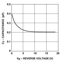
Figure 21. Typical Capacitance vs. Reverse Bias for HSMP-3860.
