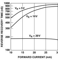
Figure 11. Typical Reverse Recovery Time vs. Reverse Voltage. HSMP-3880 Series.
