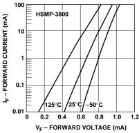
Figure 13. Forward Current vs. Forward Voltage. HSMP-3800 Series.
