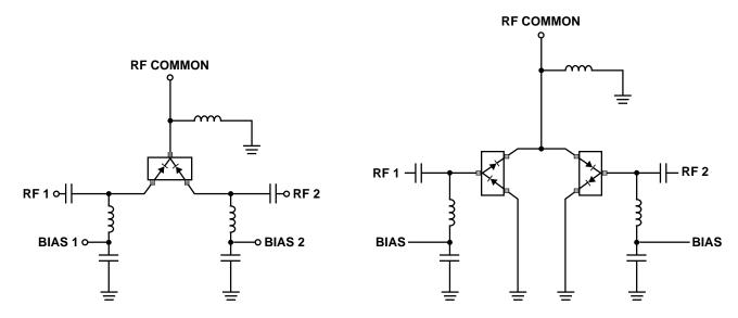
Figure 22. Simple SPDT Switch, Using Only Positive Current.
