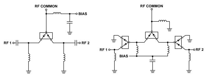
Figure 24. Switch Using Both Positive and Negative Bias Current.
