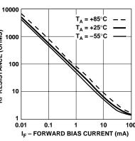
Figure 5. RF Resistance vs. Forward **Bias Current for HSMP-3810/** HSMP-4810.
