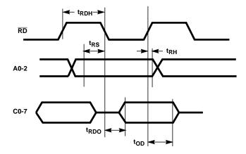
FIGURE 17. INPUT DATA TIMING
