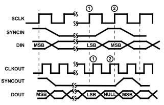
FIGURE 14A. NUMBER OF CLKOUT = NUMBER OF BITS + 1 FOR THE TIME PERIOD BETWEEN SYNCOUTS WHERE F<sub>FCLK</sub>/F<sub>SCLK</sub> = 3/2
