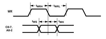
FIGURE 15. TIMING RELATIVE TO WR
