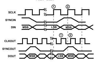
FIGURE 14B. NUMBER OF CLKOUT = NUMBER OF BITS FOR THE TIME PERIOD BETWEEN SYNCOUTS WHERE  $F_{FCLK}/F_{SCLK} = 3/2$
