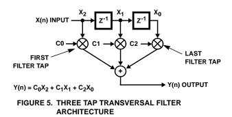
For asymmetric filters the entire coefficient set must be loaded. The coefficients are loaded in order starting with the first tap and ending with the final filter tap (see Figure 5 for tap/coefficient association). Enough storage is provided for a 128 tap asymmetric filter. For asymmetric filters the value loaded into the Programmable Filter Length Register addressed must be twice the actual number of coefficients.
