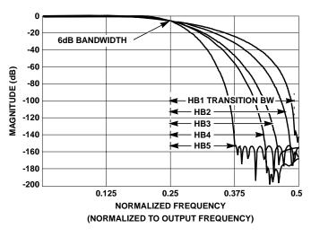
FIGURE 10C. COMPOSITE RESPONSE OF FIXED COEFFI-CIENT HALFBAND FILTERS WITH RESPECT TO THE NORMALIZED FREQUENCY SHOWN IN FIG-URE 10A
