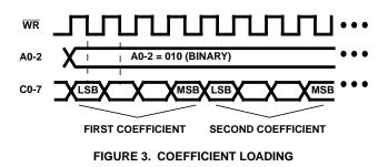
The number of coefficients that must be loaded is dependent on whether the coefficient set exhibits even symmetry, odd symmetry, or asymmetry (see Figure 4).
