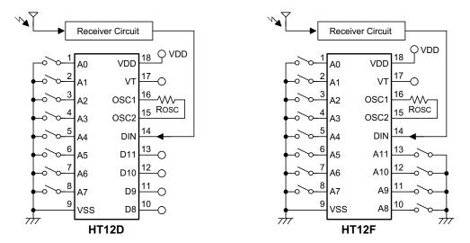
Notes: Typical infrared receiver: PIC-12043T/PIC-12043S (KODESHI CORP.) or LTM9052 (LITEON CORP.)
