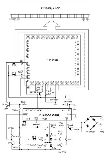
$<sup>^{\</sup>star}$  The IC substrate should be connected to VDD in the PCB layout artwork.
