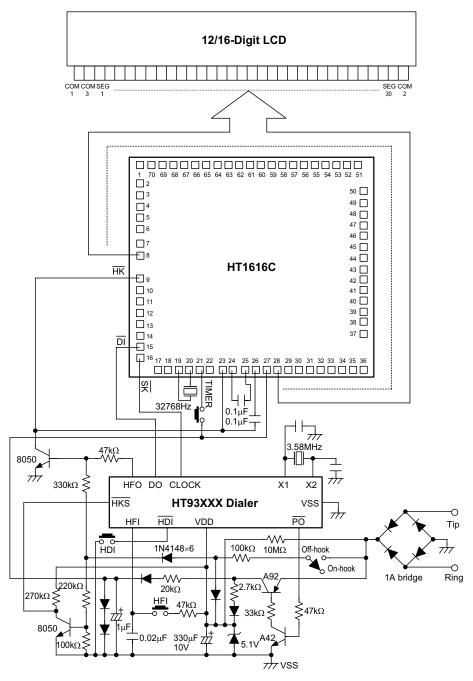
$^{\star}$  The IC substrate should be connected to VDD in the PCB layout artwork.
