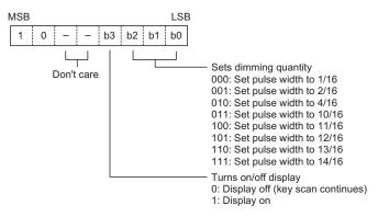
Note: power-on status: 1/16 pulse width is set and the display is turned off. Key scanning will be stopped during power-on status.
