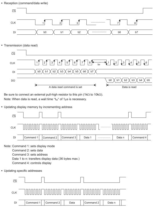
Note: Command 1: sets data Command 2: sets address Data: display data
