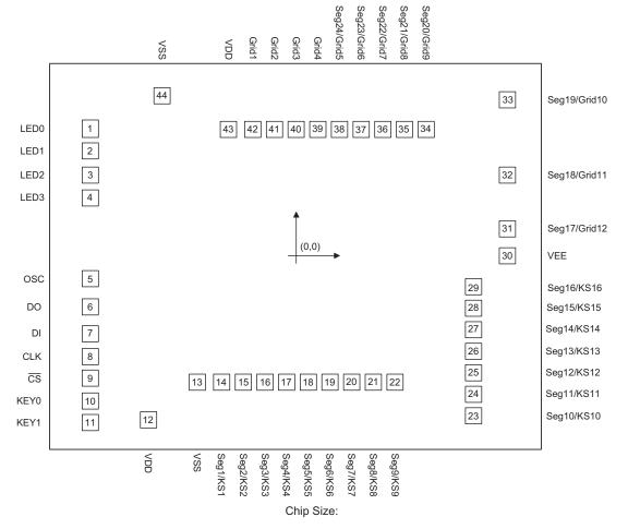
$^{\ast}$  The IC substrate should be connected to VSS in the PCB layout artwork.
