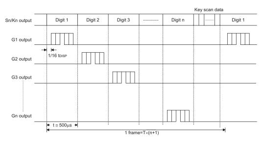
Note: One cycle of key scanning consists of two frames, and data of 16×2 matrixes is stored in the RAM.
