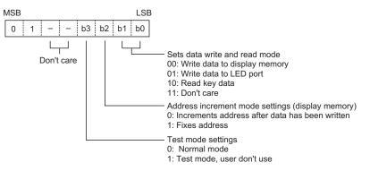
Note: power-on status: normal mode operation and address increment mode are set.
