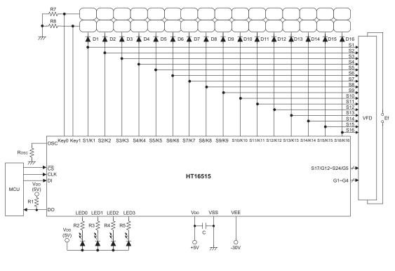
Note:  $R_{OSC}$ =82k $\Omega$  for oscillator resistor R1=1~10k $\Omega$  for external pull-high resistor R2~R6=750 $\Omega$ ~1.2k $\Omega$ R7~R8=10k $\Omega$  for external pull-low resistor D1~D6=1N4001 Ef=Filament voltage for VFD C=0.1 $\mu$ F~1.0 $\mu$ F
