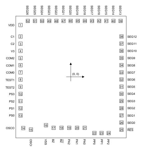
\* The IC substrate should be connected to VSS in the PCB layout artwork.
