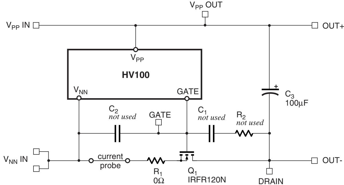
A very high dV/dt on the input can overload the HV100's internal gate clamp, causing turn-on transients. A capacitor in the  $C_2$  position may be used to clamp the gate, preventing the transients. A 1nF value is usually adequate. Voltage rating should be 16 volts.
