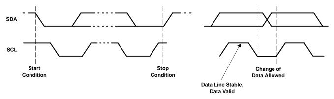
Figure 3–7. Serial-Bus Start/Stop Conditions and Bit Transfers
