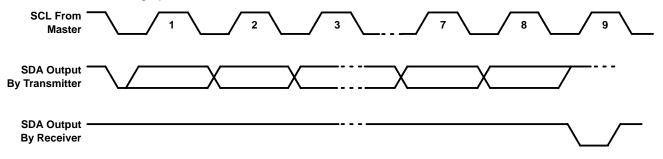
Figure 3–8. Serial-Bus Protocol Acknowledge
