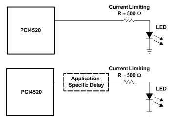
Figure 3–6. Two Sample LED Circuits
