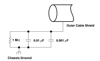
Figure 3–17. Typical Compliant DC Isolated Outer Shield Termination
