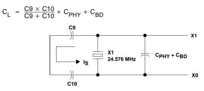
Figure 3–19. Load Capacitance for the PCI4520 PHY
