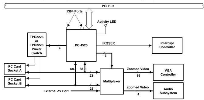
NOTE: The PC Card interface is 68 terminals for CardBus and 16-bit PC Cards. In ZV mode, 23 terminals are used for routing the ZV signals to the VGA controller and audio subsystem.
