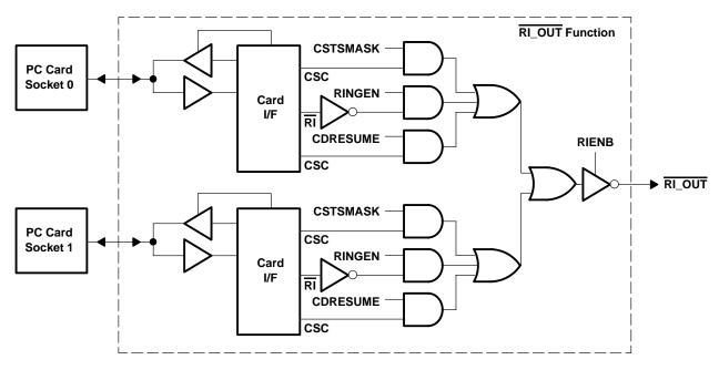
Figure 3–14. RI\_OUT Functional Diagram
