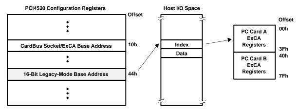
Figure 5–1. ExCA Register Access Through I/O
