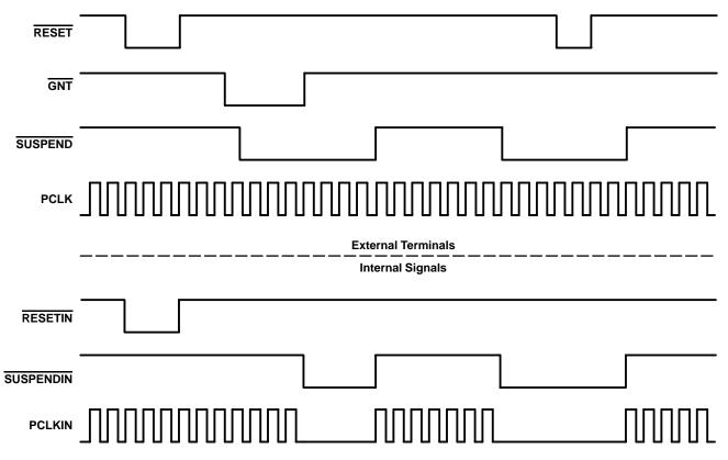
Figure 3–13. Signal Diagram of Suspend Function
