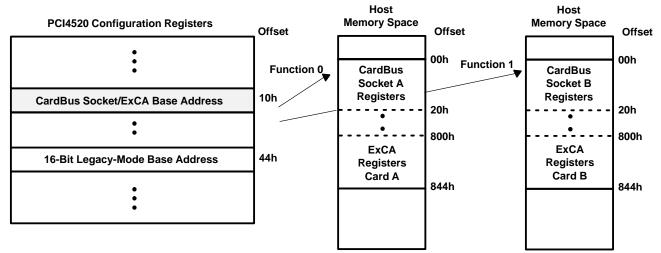
Figure 5–2. ExCA Register Access Through Memory
