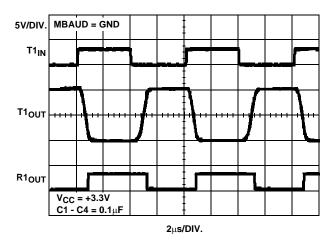
FIGURE 6. LOOPBACK TEST AT 250kbps (CL = 1000pF)
