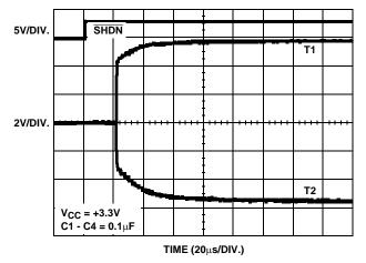
FIGURE 4. TRANSMITTER OUTPUTS WHEN EXITING POWERDOWN
