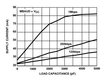
FIGURE 13. HIGH SPEED SUPPLY CURRENT VS LOAD
