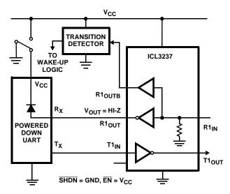
FIGURE 3. DISABLED RECEIVERS PREVENT POWER DRAIN
