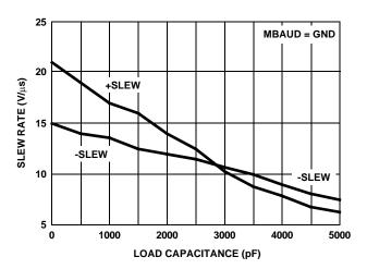
FIGURE 10. LOW SPEED SLEW RATE vs LOAD CAPACITANCE
