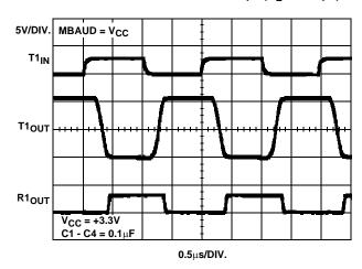
FIGURE 7. LOOPBACK TEST AT 1Mbps (C<sub>L</sub> = 250pF)
