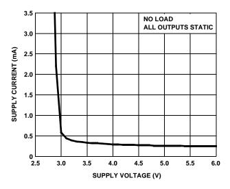
FIGURE 14. SUPPLY CURRENT vs SUPPLY VOLTAGE
