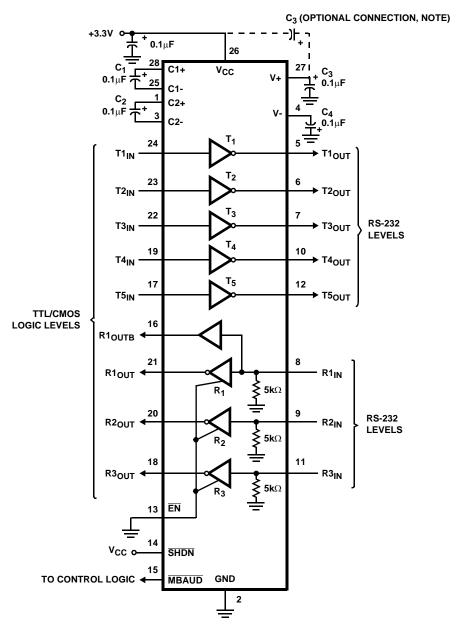
NOTE: THE NEGATIVE TERMINAL OF  $\mathrm{C}_3$  can be connected to either  $\mathrm{V}_{\mathrm{CC}}$  or gnd.
