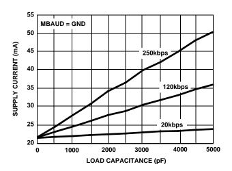
FIGURE 12. LOW SPEED SUPPLY CURRENT VS LOAD
