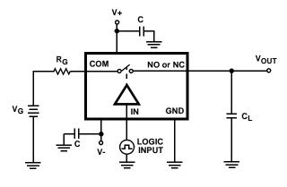
Repeat test for all switches.  $\rm C_L$  includes fixture and stray capacitance.
