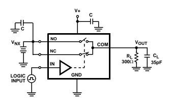
Repeat test for all switches.  $\mathbf{C}_{\boldsymbol{\mathsf{L}}}$  includes fixture and stray capacitance.
