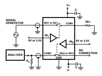
FIGURE 6. CROSSTALK TEST CIRCUIT
