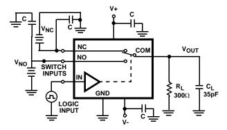
Repeat test for all switches. CL includes fixture and stray capacitance.  $\hfill \hfill \hfi$
