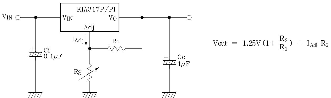
C<sub>i</sub> is required when regulator is located an appreciable distance from power supply filter.
