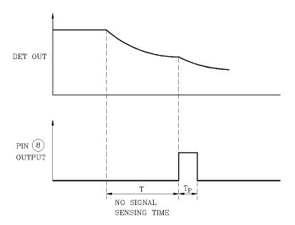
The output pulse width is measured as  $T_{\mbox{\scriptsize P}}$
