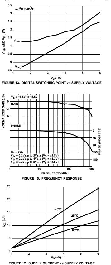
**Typical Performance Curves**  $T_A = 25^{\circ}C$ ,  $V_{IH} = V_{+}$ ,  $V_{IL} = 0V$ , Unless Otherwise Specified (Continued)
