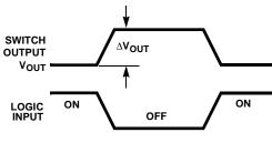
FIGURE 2A. MEASUREMENT POINTS
