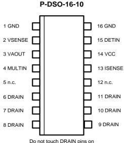
Do not touch DRAIN pins on application board: 650V
