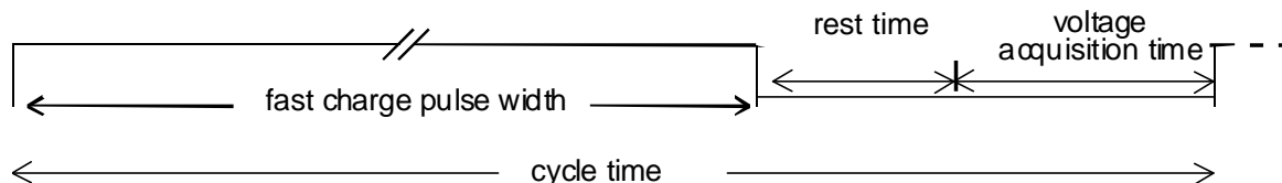
Figure 4: Charge cycle showing fast charge current pulses
