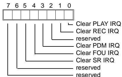
This register provides the driver software easy access to the interrupt source when read. Note that bit 7 indicates the state of the IRQ pin, and hence will be zero when the MIE bit is zero (see "Interrupt Enable" register).
