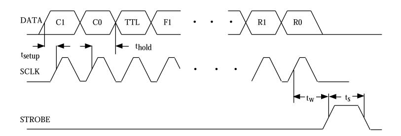
Figure 2. Timing Diagram for Programming the ICS307
