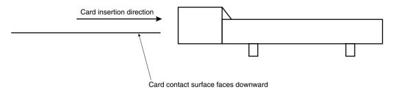
2. After the smart card has been inserted, be sure not to appy excessive force to the card portion that protrudes from the insertion slot.
