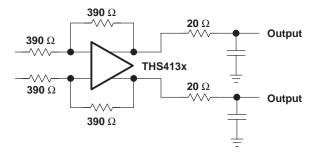
Figure 33. Driving a Capacitive Load
