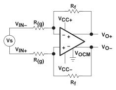
Note: For proper operation, maintain symmetry by setting  $R_f 1 = R_f 2 = R_f$  and  $R_{(g)} 1 = R_{(g)} 2 = R_{(g)} \Rightarrow A = R_f/R_{(g)}$
