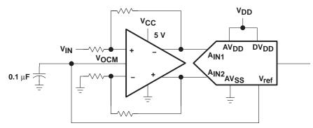
Figure 31. Fully Differential Amplifier Using a Single Supply
