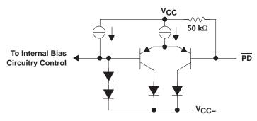
Figure 41. Simplified Power-Down Circuit
