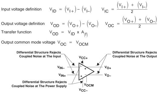
Figure 36. Definition of the Fully Differential Amplifier
