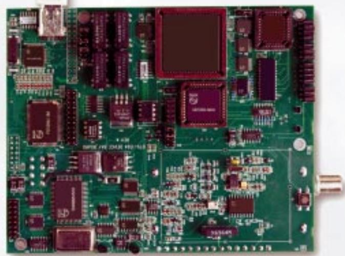
One of the key chips in the Device Bay module, the TDA8960 accepts 8-VSB modulated signals from the IF block of the tuner front-end, or alternatively, the VSB IC AGC control output can be applied directly to the tuner. Adaptive equalization using the ATSC field sync (trained equalization) and/or the 8-VSB data itself (blind equalization) is performed via a decision feedback equalizer (DFE) following internal carrier recovery, half Nyquist filtering and symbol timing recovery.
