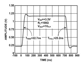
FIGURE 13. LARGE SIGNAL STEP RESPONSE
