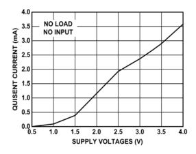
FIGURE 12. SUPPLY CURRENT vs SUPPLY VOLTAGE
