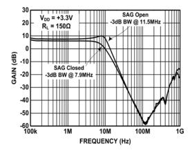
FIGURE 3. GAIN vs FREQUENCY -3dB
