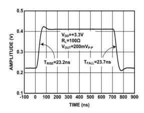
FIGURE 14. SMALL SIGNAL STEP RESPONSE
