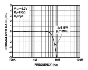
FIGURE 2. GAIN vs FREQUENCY -3dB POINT
