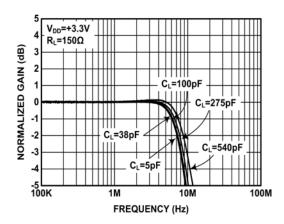
FIGURE 5. GAIN vs FREQUENCY FOR VARIOUS  $C_{\mbox{LOAD}}$
