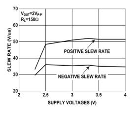
FIGURE 21. SLEW RATE vs SUPPLY VOLTAGE
