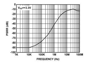
FIGURE 8. PSRR vs FREQUENCY
