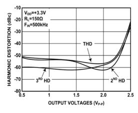
FIGURE 18. HARMONIC DISTORTION vs OUTPUT VOLTAGE
