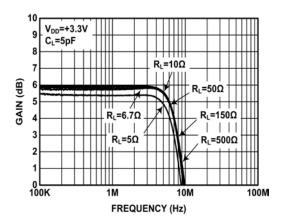
FIGURE 4. GAIN vs FREQUENCY FOR VARIOUS  $R_{\mbox{\scriptsize LOAD}}$
