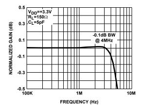
FIGURE 1. GAIN vs FREQUENCY -0.1dB
