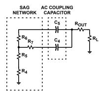
FIGURE 25. SAG NETWORK AND AC COUPLING CAPACITORS
