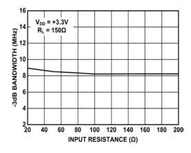
FIGURE 20. -3dB BANDWIDTH VERSUS INPUT RESISTANCE
