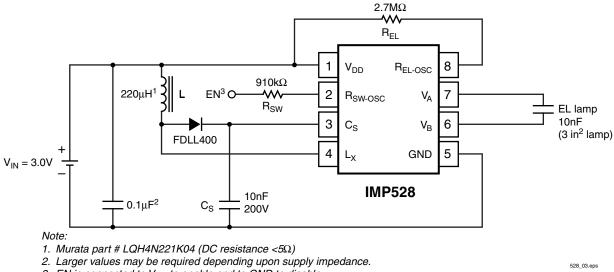
3. EN is connected to  $V_{DD}$  to enable and to GND to disable.
