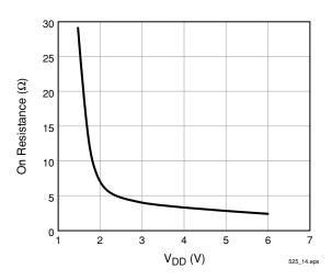
Figure 6. Boost Switch On Resistance
