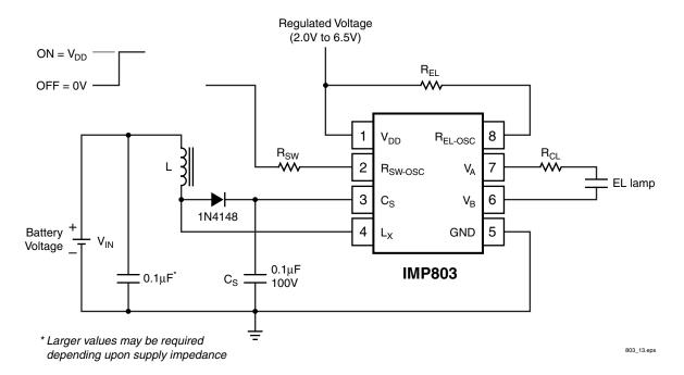
Figure 5. Dual Supply Operation
