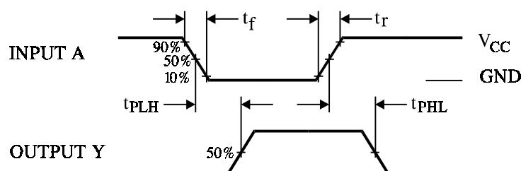
Figure 1. Switching Waveforms
