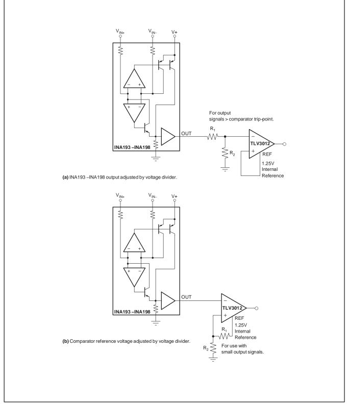
Figure 10. INA193-INA198 With Comparator
