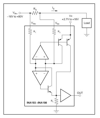
Figure 1. INA193-INA198 Basic Connection
