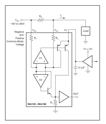
Figure 4. INA193-INA198 Example Shutdown Circuit
