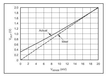
Figure 2. Example for Low V<sub>SENSE</sub> Cases 1 and 3 (INA195, INA198: Gain = 100)
