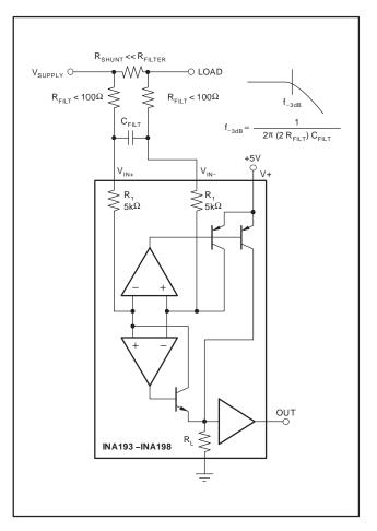
Figure 5. Input Filter (Gain Error – 1.5% to –2.2%)
