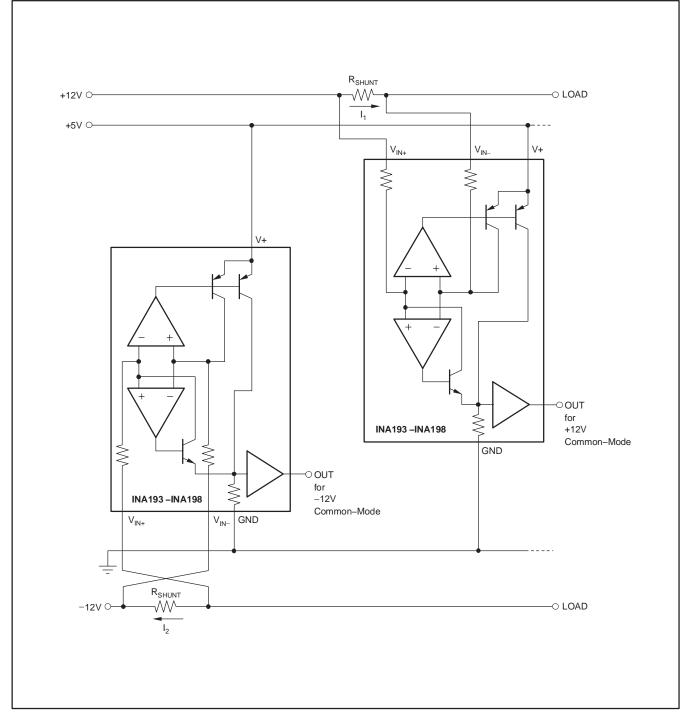
Figure 7. Monitor Bipolar Output Power-Supply Current
