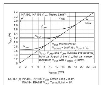
Figure 3. Example for Low V<sub>SENSE</sub> Case 2 (INA195, INA198: Gain = 100)
