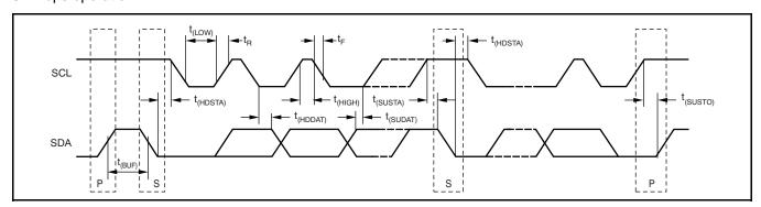
Figure 20. Bus Timing Diagram
