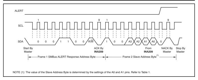
Figure 18. Timing Diagram for SMBus ALERT
