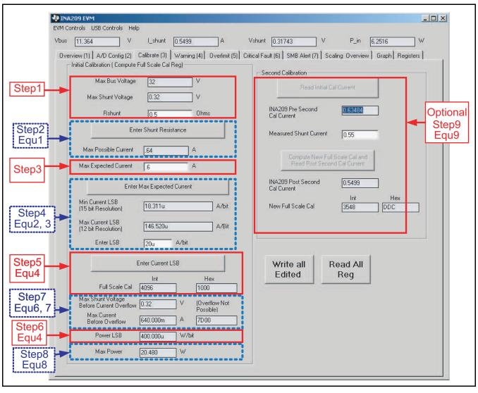
Figure 25. INA209 Calibration Sofware Automatically Computes Calibration Steps 1-9
