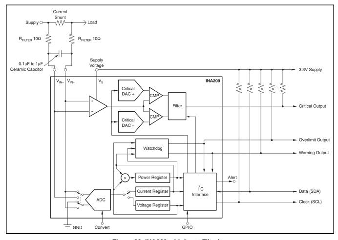
Figure 22. INA209 with Input Filtering
