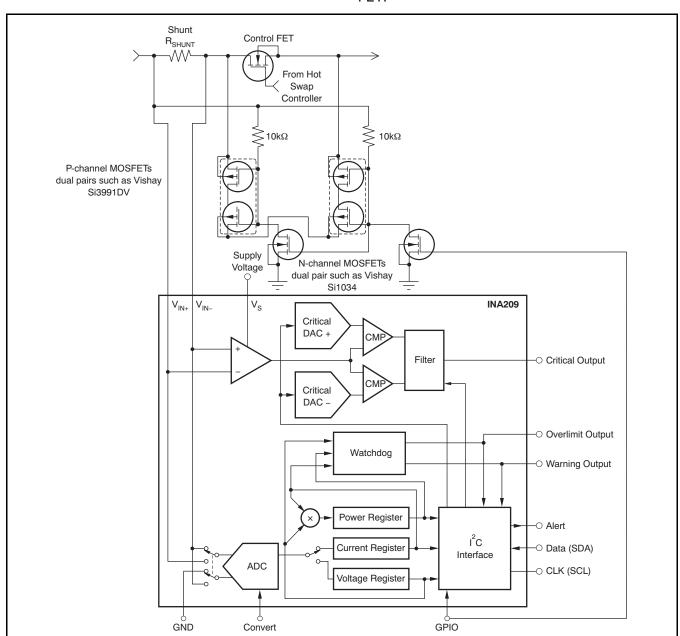
Figure 24. External Circuitry for Additional V<sub>BUS</sub> Input
