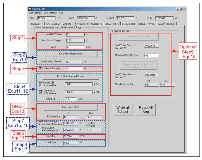
Figure 26. Calibration Software Automatically Computes Calibration Steps 1-9
