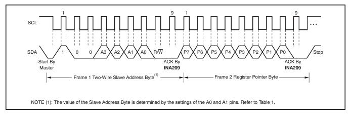
Figure 19. Typical Register Pointer Set
