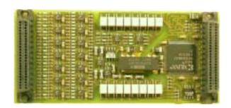
All inputs have an electronic debounce circuit. The debounce time is programmable in a range from 900µs up to 230ms in 256 steps of 900µs. The debounce circuit can also be disabled. The TIP606 is designed for an operating temperature from -40°C to +85°C.
