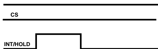
FIGURE 7. POWER UP SEQUENCE
