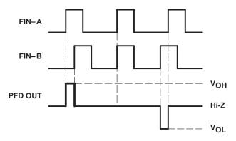
Figure 2. PFD Function Timing Chart
