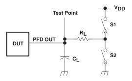
Figure 5. PFD Output Test Conditions
