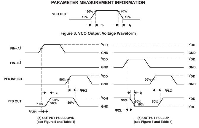
$^{\dagger}$  FIN–A and FIN–B are for reference phase only, not for timing.
