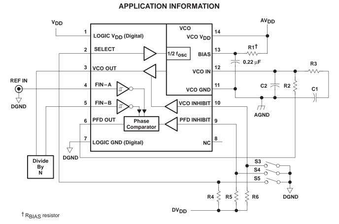
Figure 28. Evaluation and Operation Schematic
