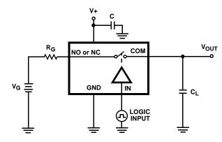
FIGURE 2A. MEASUREMENT POINTS
