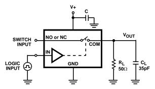
Repeat test for all switches. C<sub>L</sub> includes fixture and stray capacitance.
