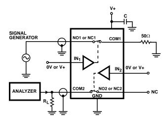
FIGURE 5. CROSSTALK TEST CIRCUIT
