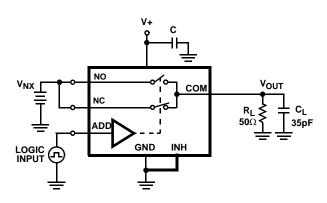
Repeat test for all switches.  $\mathbf{C}_{\mathsf{L}}$  includes fixture and stray capacitance.
