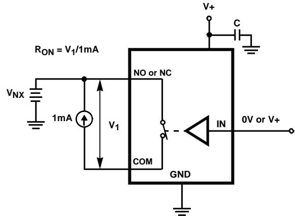
FIGURE 5.  $R_{ON}$  TEST CIRCUIT
