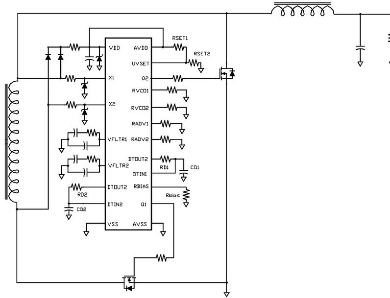
Fig. 1 Typical application circuit when supply  $V_{out} < 5.0 V_{DC}$
