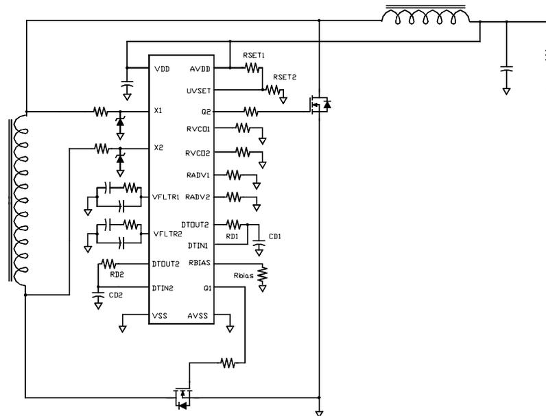
Fig. 2 Typical application circuit when supply  $V_{out} = 5.0 V_{DC}$
